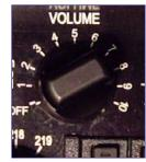
As with any receiver, you want to avoid overdriving it. This happens when you turn up the **Volume** too far. Overdriving doesn't hurt the digital Field Marshall, but makes it so you get the same signal in every direction, (sometimes the signal may actually decrease in the direction of the transmitter.)
