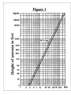
This diagram can give you an idea of the line-of-sight distance. To use it compute the distance for the height of the transmitter and your own height separately, then add them together. For example, if your transmitter was on a hill 25 feet high and your receiver was 8 feet high, the line-of-site distance would be 11 miles (7 + 4 miles).
