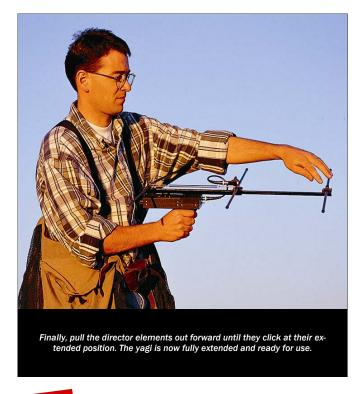
The antenna won't give its best range and pin-point accuracy **unless** fully deployed as shown in the picture above.
