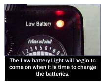
Actual battery life depends on many factors, including temperature and how long it is used continuously. All batteries will run longer if used for short periods of time with time to rest in between (rather than continuously with no rest.)
