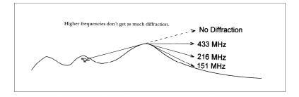
It is important to remember that the frequency is very important. Higher frequency means less diffraction. Higher frequency transmitters may perform equally well at close range on flat ground, but will not do well at a distance or in hilly terrain. This is unfortunate, because higher frequencies allow smaller antennas. The frequency of your Marshall receiver, between 173 and 220 MHz gives a good compromise between antenna size and ground-hugging (diffraction) ability.
