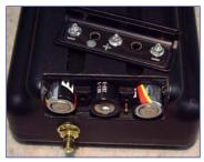
**Caution:** Please observe the battery polarity as shown in the picture and marked on the battery cover lid – negative on the two sides and positive in the middle.
