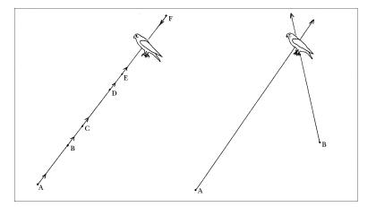
the exact location of the transmitter: at the intersection of the two lines. You probably can't follow the line to the transmitter directly anyway because of roads and obstacles or the need to stay on high ground, so take advantage of that fact.
