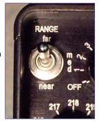
**Note:** Other receivers have powerful Medium settings which tend to fool you into thinking a transmitter is closer than it is. This high sensitivity is good on Far, but on Medium, this is *not a virtue*. The Field Marshall is intentionally designed with a weaker, and more precise Medium range.
