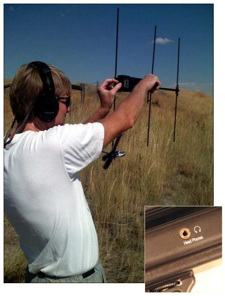
**Headphones** give a big advantage when tracking weak signals in noisy environments and are strongly recommended for serious tracking and listening to very weak signals.
