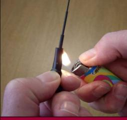
*Important*: Firmly grasp the base of the transmitter at the neck of the antenna while heating.
