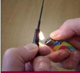
*Important*: Firmly grasp the base of the transmitter at the neck of the antenna while heating.
